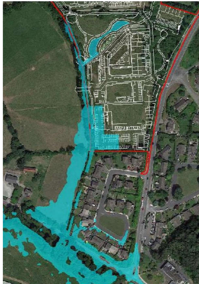
Figure 9.10: Flood mapping with proposed development (stream flow at 0.1% AEPCC, river flow at 10m 3 /s)
