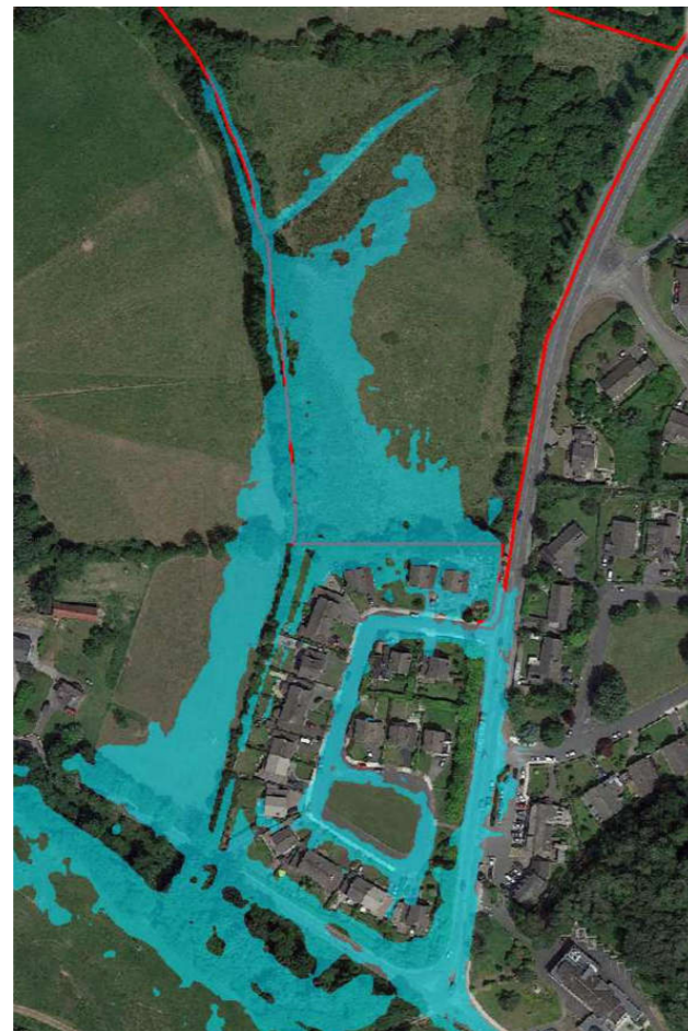
Figure 9.7: Flood mapping based on existing topography (stream flow at 0.1% AEPCC, river flow at 10m³/s)
