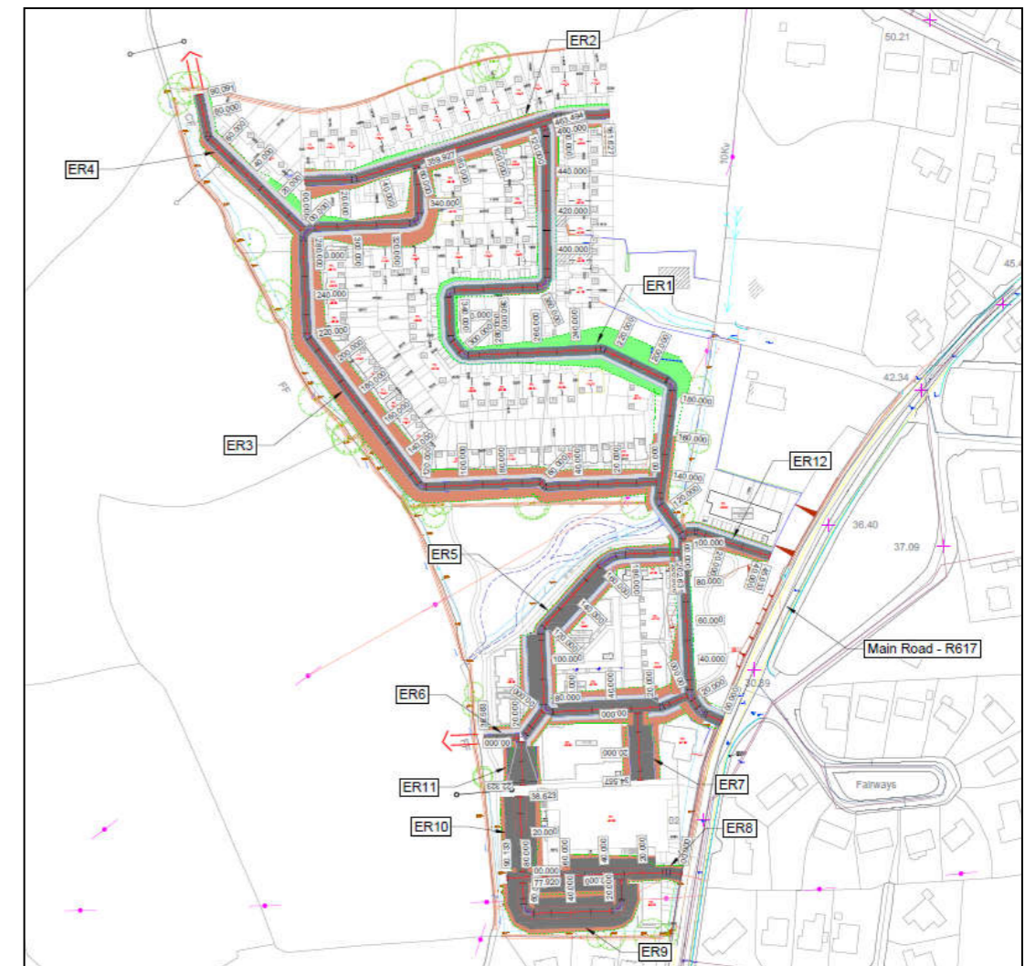
Figure 2.1: Overall proposed estate roads with cut and fill lines (refer to MHL drawing RL1-ERO-P01)
